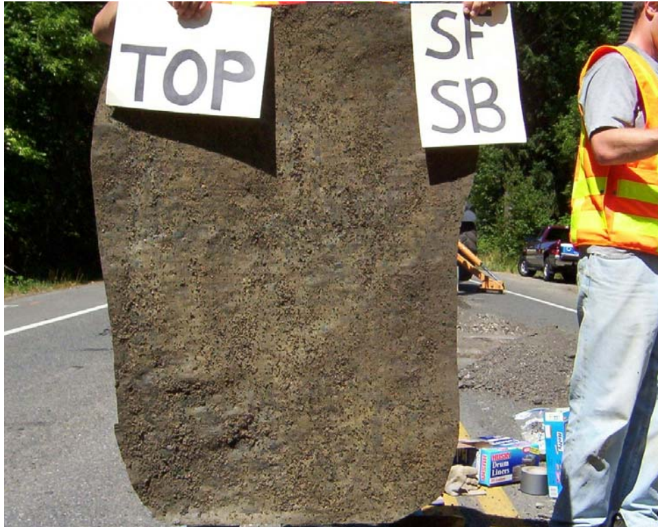
Figure 3.27. Top of SF-SB geotextile after removal.
