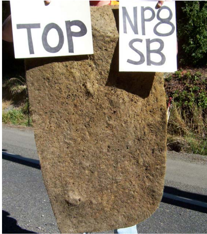
Figure 3.23. Top of NP8-SB geotextile after removal.
