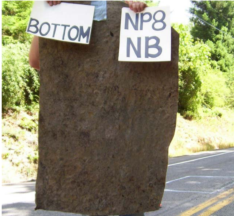
Figure 3.17. Bottom of NP8-NB geotextile after removal.
