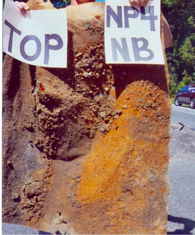
Figure 3.37. Top of NP4-NB geotextile after removal.
