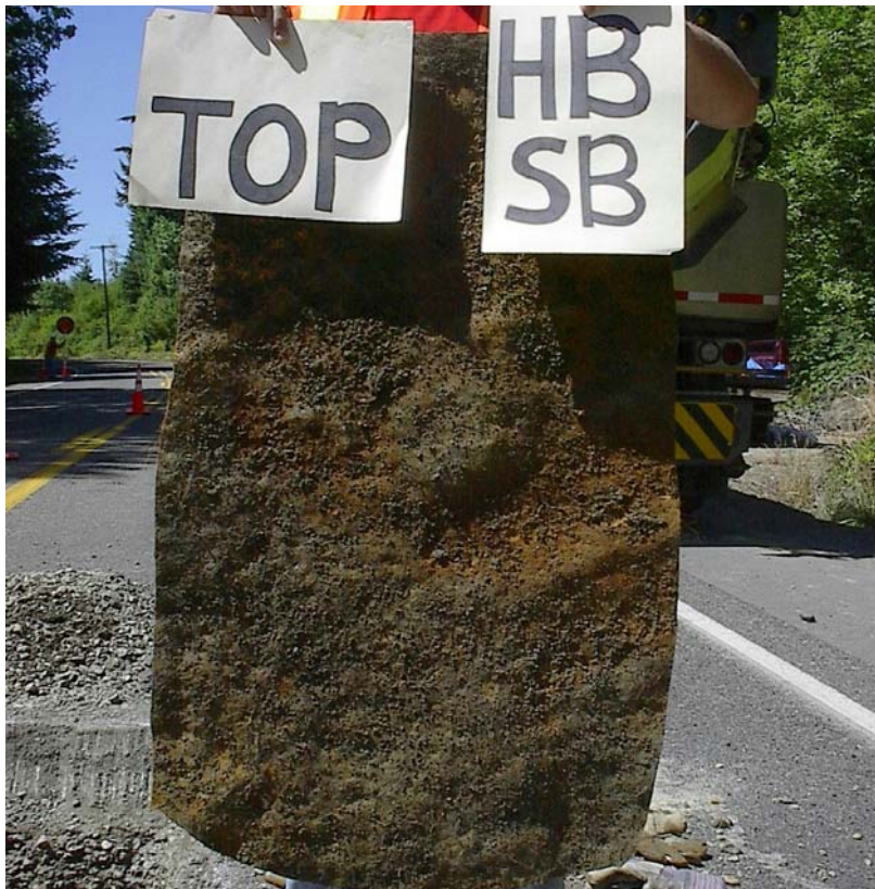
Figure 3.32. Top of HB-SB geotextile.
