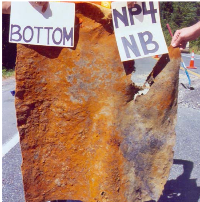
Figure 3.38. Bottom of NP4-NB geotextile after removal.
