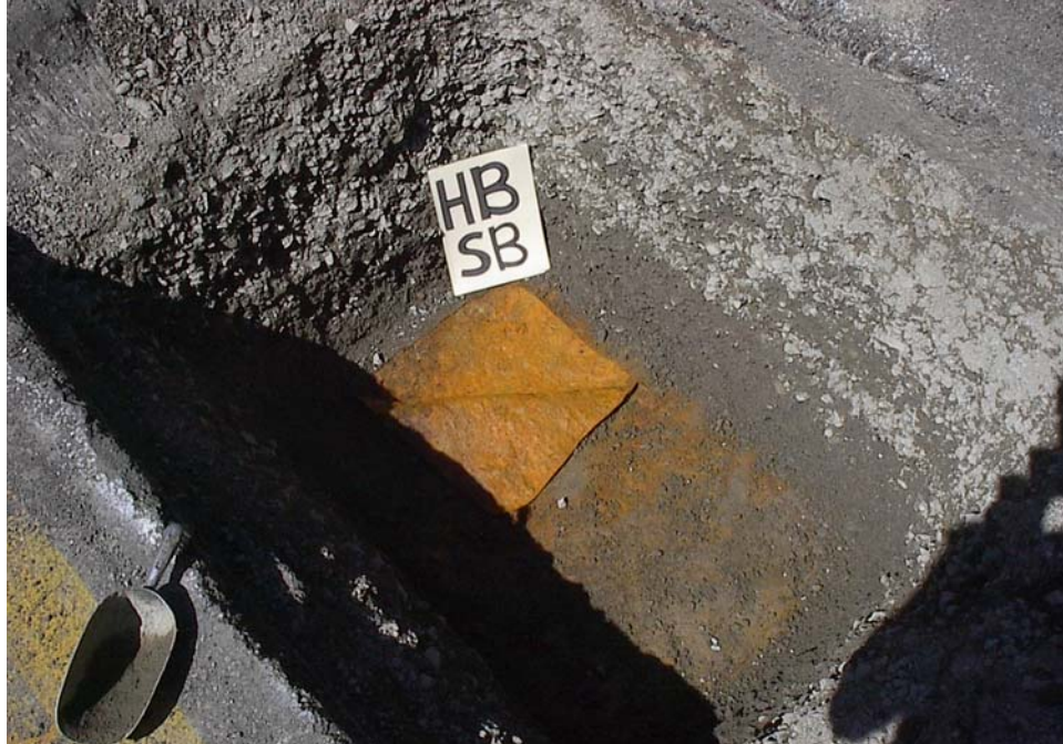
Figure 3.31. HB-SB test pit with geotextile peeled back.
