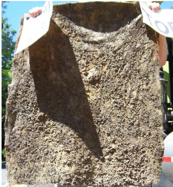
Figure 3.30. Top of NP4-SB geotextile after removal.
