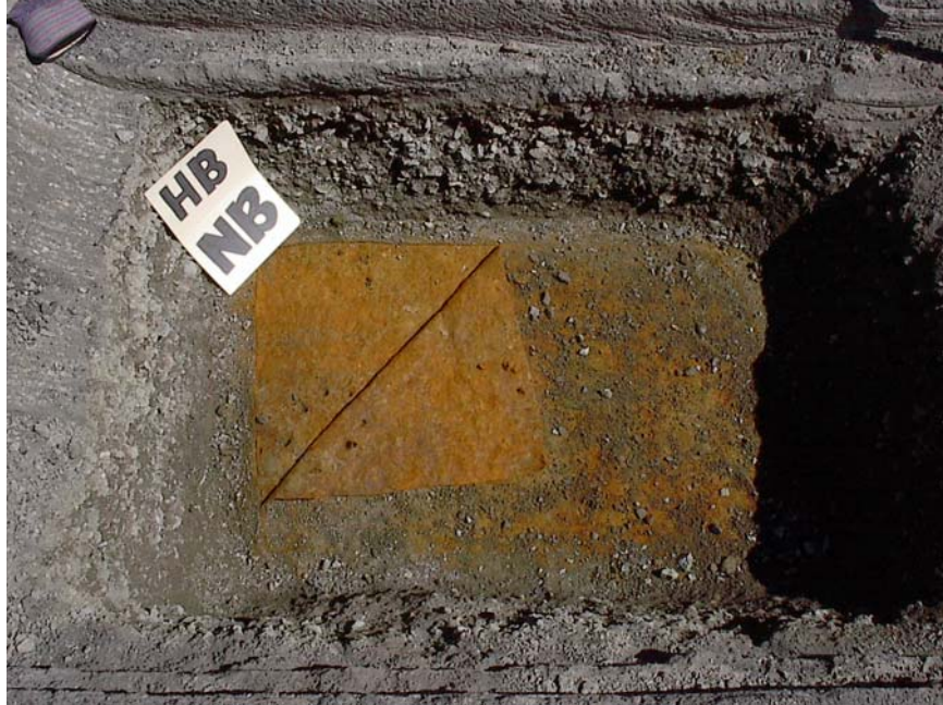
Figure 3.39. HB-NB test pit with geotextile peeled back.
