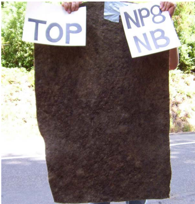
Figure 3.18. Top of NP8-NB geotextile after removal.
