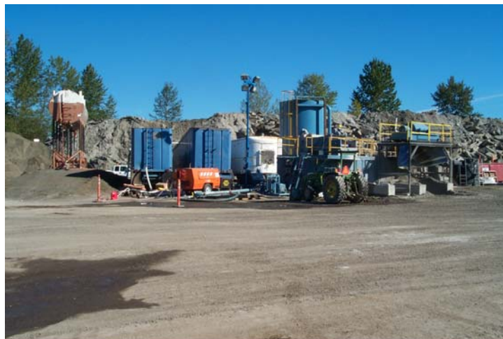
Photo 41. Processing plant for treating diamond grinding slurry.
