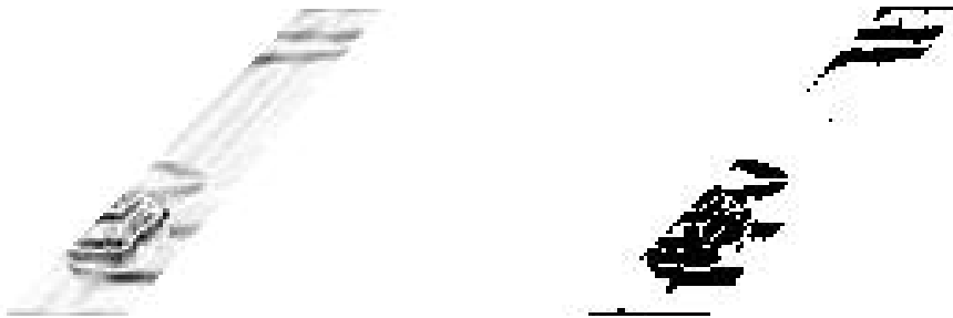
Figure 101. a) Horizontal image gradient features found in a lane of uncongested traffic. b) Binary edge features remaining after thresholding.
