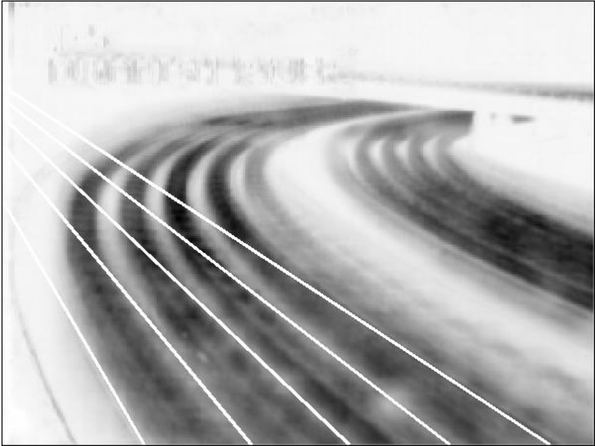
Figure 59. Lane boundaries found with the proposed algorithm superimposed on the activity map.
