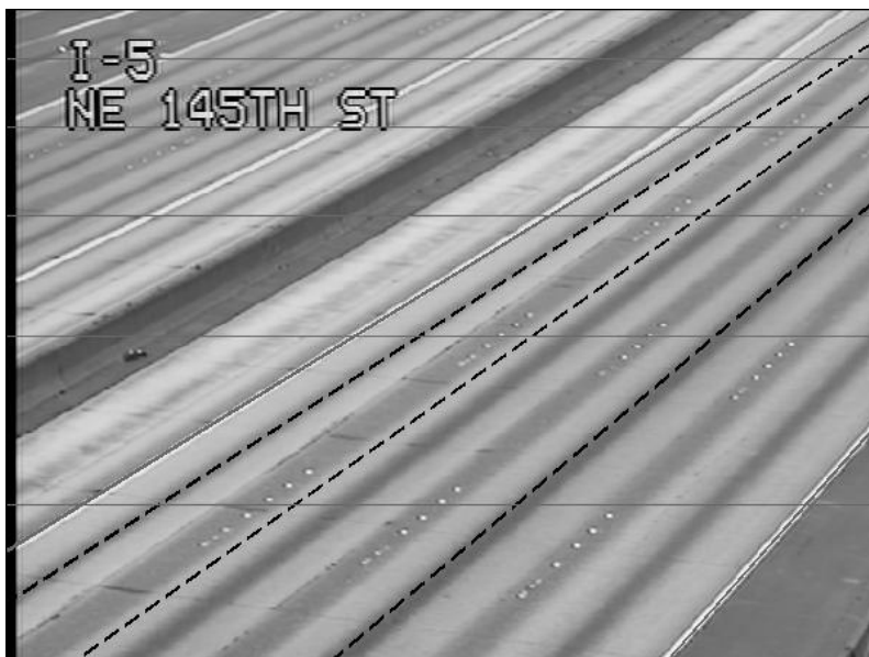
Figure 97. Background image for the sequence of Figure 94(c). The road boundaries are marked with solid lines, and the lane boundaries are marked with dashed lines. The 40-foot intervals are marked with horizontal lines.
