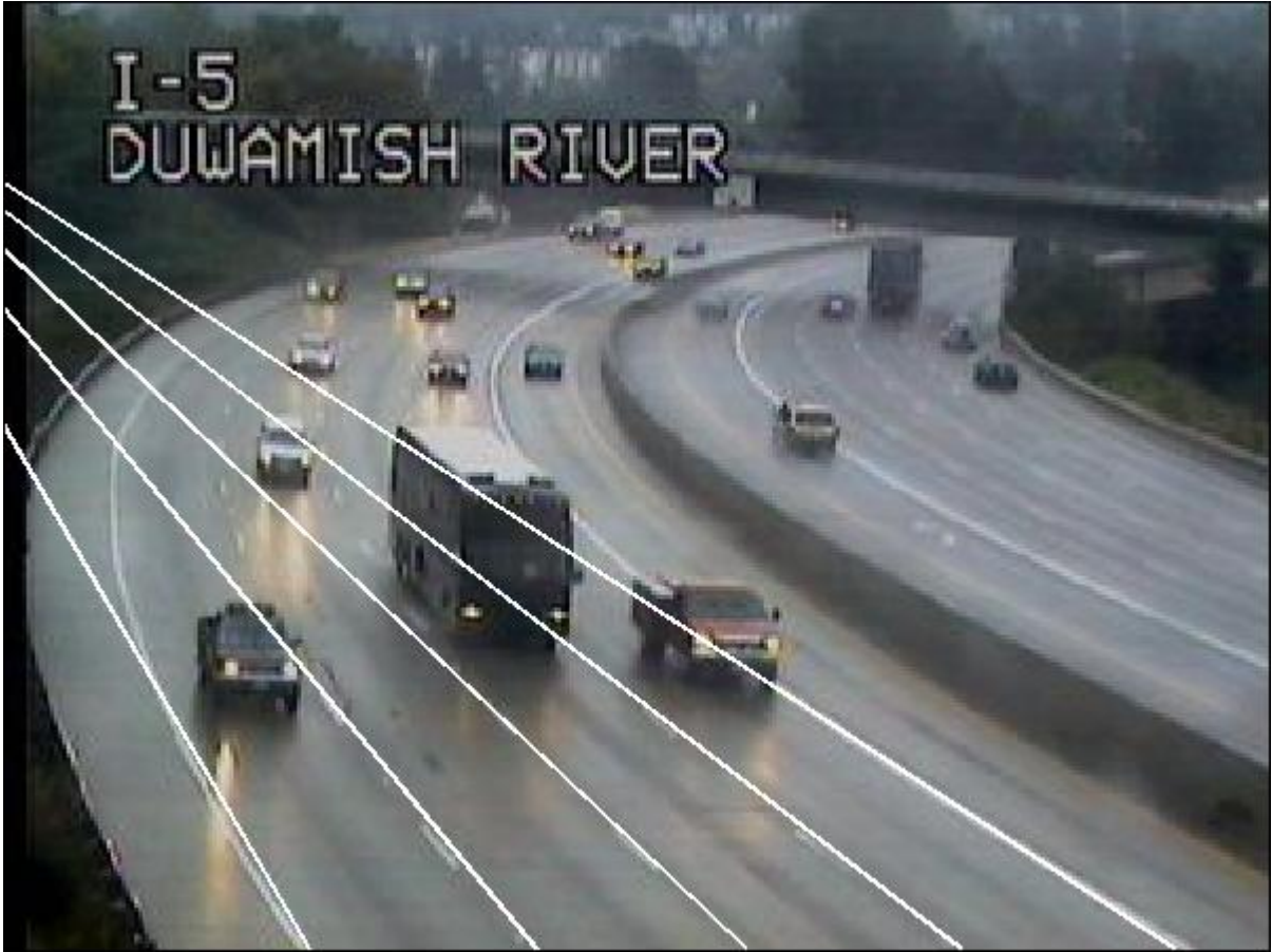
Figure 60. Lane boundaries found with the proposed algorithm superimposed on an image of the scene.
