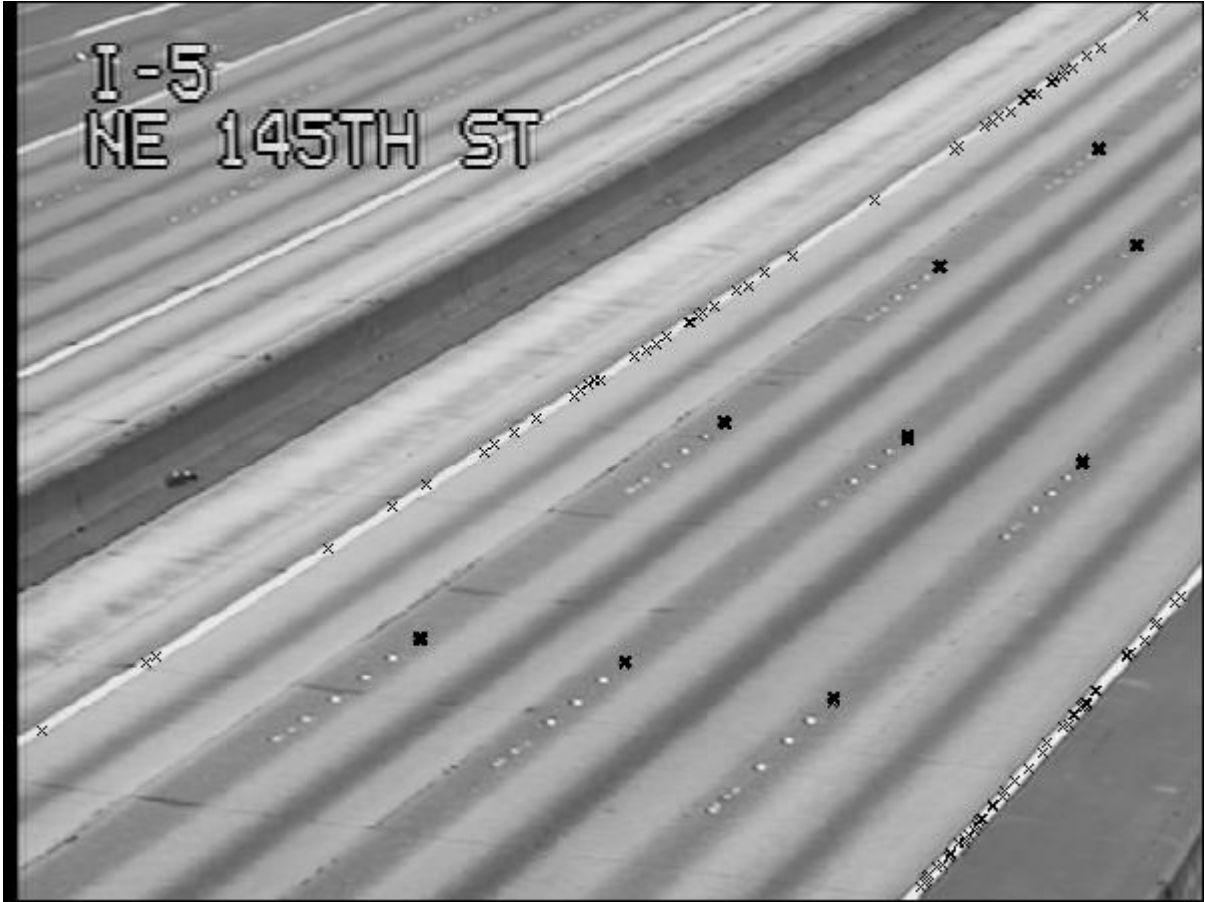
Figure 89. Sample image used in hand-calibration of the camera with superimposed points clicked by a human observer.
