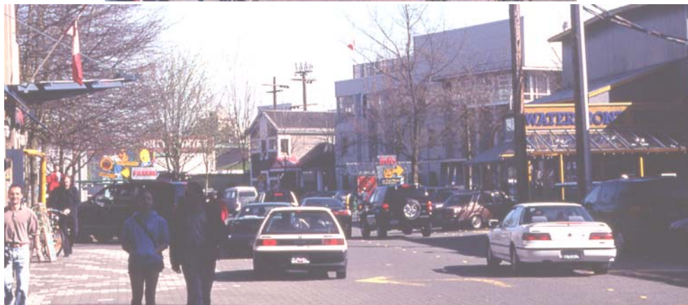
Figures IV.5 and IV.6: Granville Island, Vancouver, B.C. On-street parking slows traffic, creates better pedestrian environments by buffering sidewalks from moving vehicles, increases the viability of retail shops and services, and contributes to reducing the amount of land used for off-street lots.
