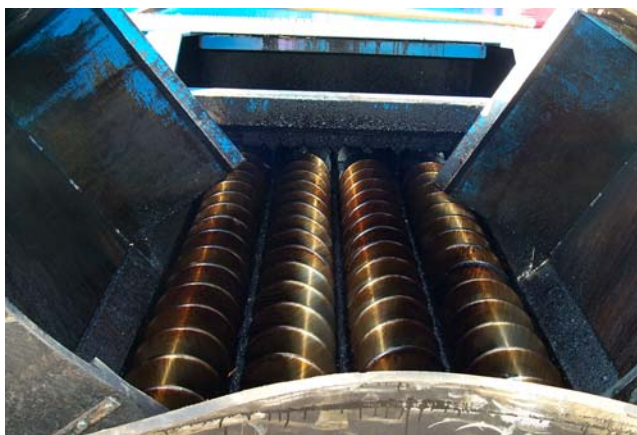
Photo 19. Auger system within the Novapaver.
