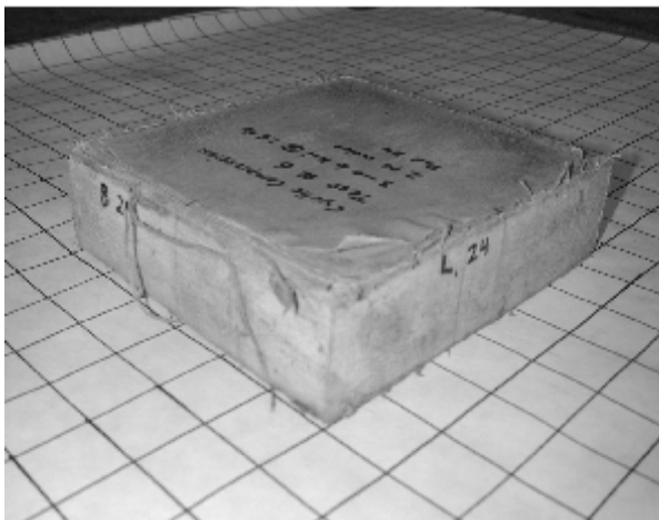
c) Category C - Delamination
