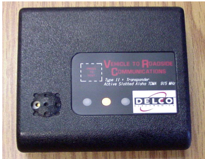
Figure 14. Typical Truck Windshield Transponder
