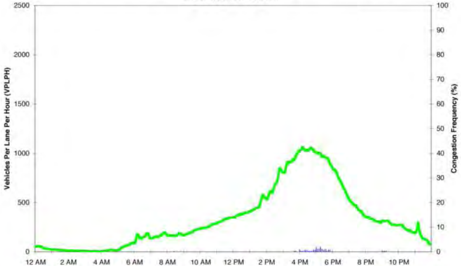
Figure 4.20. Estimated Weekday Volume, Speed, and Reliability Conditions (2001): Southbound SR 167, South 34th St, HOV Lane
