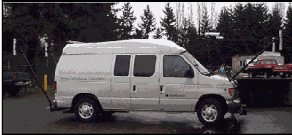
Figure 7. WSDOT Pavement Distress Identification Van
