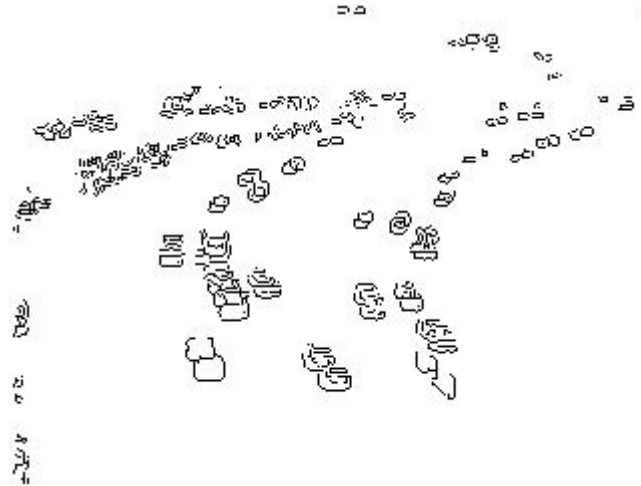
Figure 2.4 Sobel edges in the difference image between the first two frames
