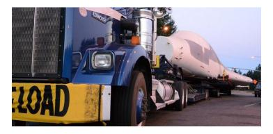
Superload truck freight example; Boeing B1 bomber 131 feet long, 29+ feet wide, and 15 feet high.
