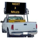
Truck-mounted PCMS displays two messages for 2 second each of a work zone queue ahead.
