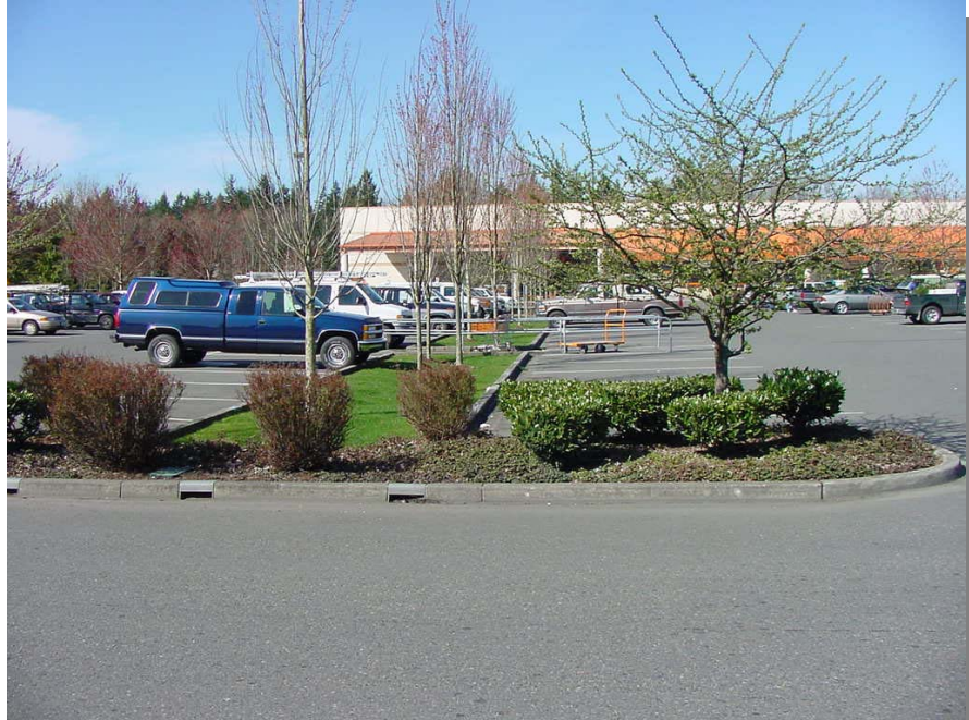
Figure 630.5 Vegetated bioswale in parking lot
