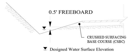
Ditches should not be confused with biofiltration swales. In addition to collecting and conveying drainage, biofiltration swales also provide runoff treatment by filtering out sediment. (See the *Highway Runoff Manual* for design guidance for biofiltration swales.) Roadside ditches are to be designed so the integrity or geometry of the roadway is not compromised.
