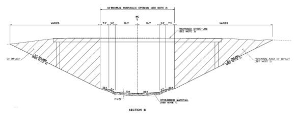
There are three methods for determining the minimum hydraulic opening: stream simulation, confined bridge, and unconfined bridge. However, the process used for confined bridge is the same as stream simulation. All methods are dependent on the floodplain utilization ration (FUR), which determines how confined a stream is. The minimum hydraulic opening is determined from Equation 7-1 (2013 WCDG, Equation 3.2), unless otherwise approved by the HQ Hydraulics Section.
