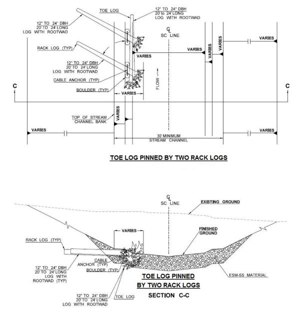
Figure 10C-2 Toe Log Pinned by Two Rack Logs
