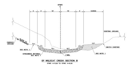
Flows within the channel cross section must mimic those in the reference reach. For example, if the active channel is overtopped at less than a 2-year event, the channel should behave the same through the design reach.
