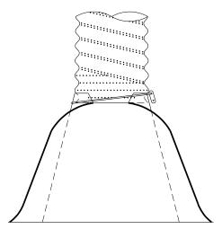
A flared end section is usually the most feasible option in smaller pipe sizes and should be considered for use on culverts up to 48 inches in diameter. For diameters larger than 48 inches, end treatments such as concrete headwalls tend to become more economically viable than the flared end sections.
