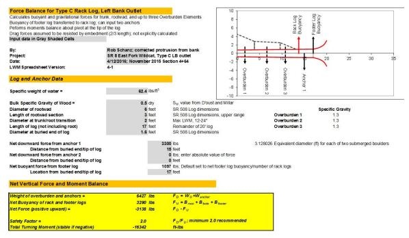
The three-log structures require a more complex stability analysis that accounts for the transfer of forces between the footer log and the overlying rack logs. Figure 10A-3 illustrates the free body diagram and calculations for one of the rack logs in these structures. We assumed the footer log buoyancy will be transferred equally to each of the two rack logs. The factor of safety for vertical buoyancy forces for each rack log is then:
