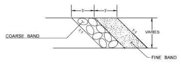
Coarse bands are required within all structures that are four sided and that have a stream slope of 2 percent or less. Coarse bands are recommended within all structures that have a stream slope between 2 and 4 percent. Coarse bands are typically sized for the  $D_{84}$  to be stable at the 100-year flow event and shall not have material that is larger than twice the  $D_{100}$  of the design bed mix.
