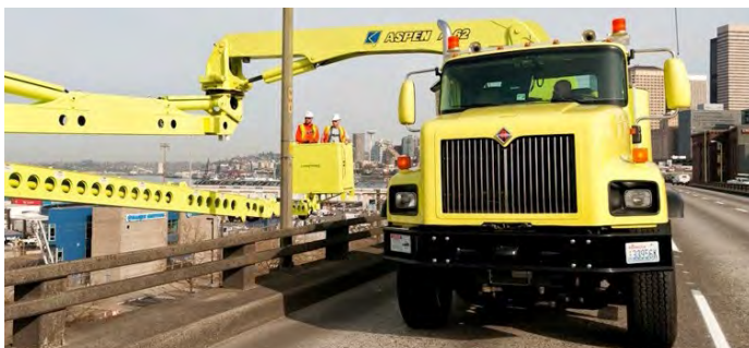
A WSDOT crew uses an Under Bridge Inspection Truck to conduct an inspection on the State Route 99 Alaskan Way Viaduct.
