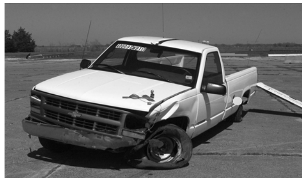
FIGURE 7 Vehicle damage – current design.
