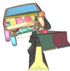
FIGURE 8 Simulation and crash test comparison – current design.
