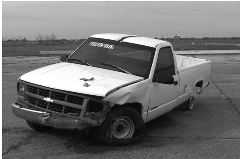
FIGURE 11 Vehicle damage – alternate design.
