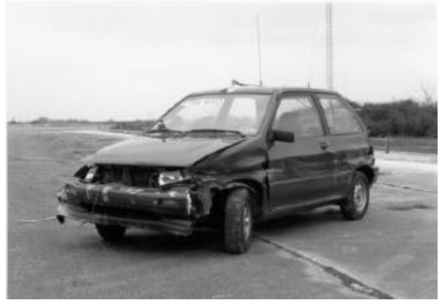
FIGURE 5 Small car damage.
