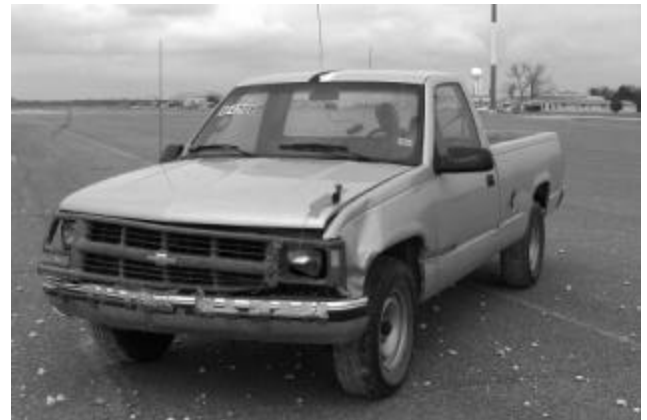
FIGURE 8 Pickup truck damage.
