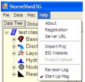
ESI Website link allows designers to access the Engenious website directly. The Import Project command can be used to import and convert old StormSHED files. It should be noted that while StormSHED files can be transferred into 3G **the layouts** created in StormSHED files can not and designers need to recreate them in 3G. The <u>Revision Log</u> will provide a list of any changes or updates that have been made to the program. If the <u>Start</u>
