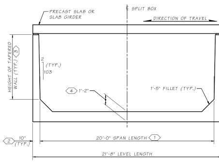
SPLIT BOX ~ SLAB SB20 DIMENSIONS FOR SBS20 SHOWN. FOR ALL OTHER SERIES REFER TO NOTES. ALL DIMENSIONS AND RELATED NOTES SHOWN ARE IN ACCORDANCE WITH BDM SECTION 8.3.6-A1-1 PRECAST FORM LIMITS.
