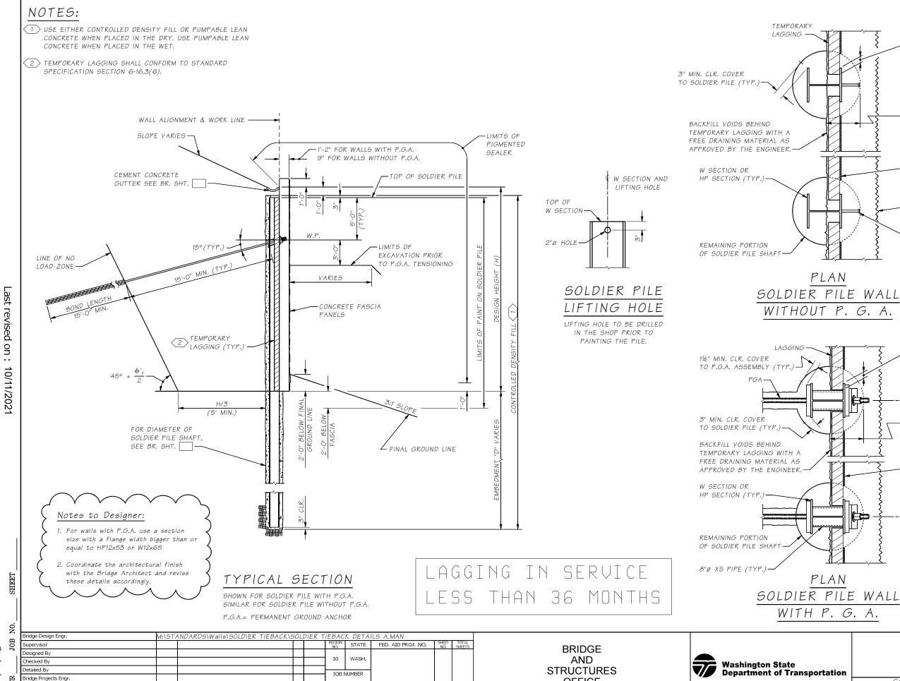
TEMPORARY 2" MIN. BEARING LENGTH SHIM AS NECESSARY FOR FULL BEARING. CHIP OUT SHAFT BACKFILL TO PLACE TEMPORARY LAGGING. 4'-0" WIDE STRIP OF PREFABRICATED DRAINAGE MAT (TYP.) CENTERED BETWEEN SOLDIER PILE FLANGES. -ARCHITECTURAL FINISH WITH PIGMENTED SEALER 34"ø x 6" WELDED SHEAR STUDS AT 1'-0" (TYP.) PLAN
