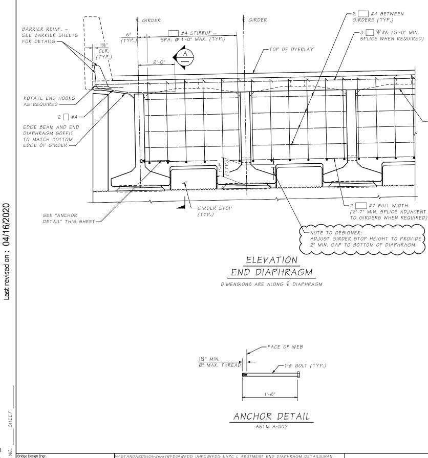
NOTE TO DETAILER: DIAPHRAGM Revise Details to show correct BRG. -OPTIONAL FIELD ₩#6 (TYP.) BEND (TYP.) SEE EXPANSION JOINT, EDGE BEAM AND ABUTMENT -TOP OF OVERLAY DETAILS ON BRIDGE SHEETS TOP OF GIRDER GRADE\_\_ #4 AT EXT. GIRDERS 1'-0" MAX. #4 BETWEEN GIRDERS (TYP.) EDGE BEAM #4 STIRRUP SOFFIT-END OF GIRDER € DIAPHRAGM NORMAL TO GIRDER BOTTOM BEARING PAD -INTERSECTION OF € DIAPHRAGM & & BEARING SECTION LONGITUDINAL DIMENSIONS ARE NORMAL TO DIAPHRAGM. GIRDER STOP NOT SHOWN FOR CLARITY.
