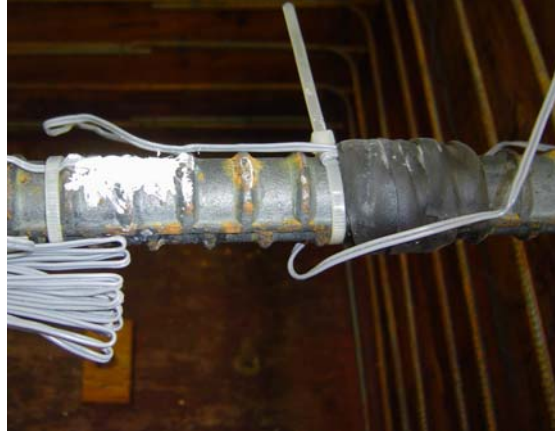
Figure 3-13. Two gauges at different stages of protecting (Picture courtesy of Jason Pang).
