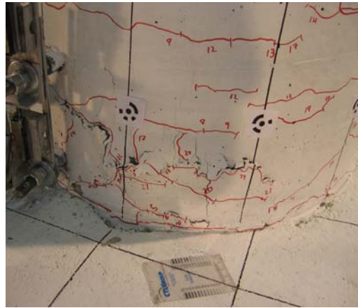
Figure 4-5. LB7-PT: north side, Cycle 24 (2.26%).
