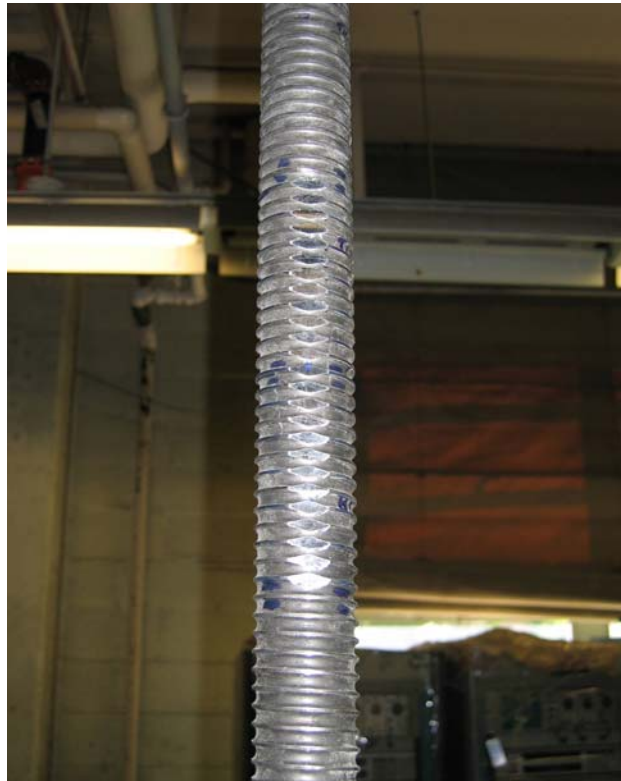
Figure B-8. PT bar used in tension test.
