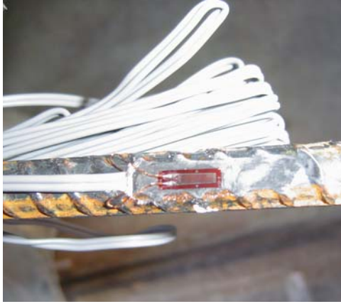
Figure 3-12. Strain gauge after gluing (Picture courtesy of Jason Pang).
