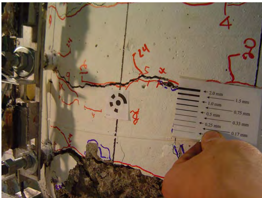
Figure 4-6: Crack localization in Specimen DB5-RE at Cycle 25 (2.96%/-3.02)
