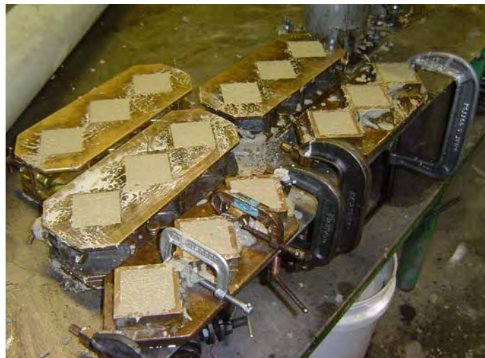
Figure B-15: Molding of grout cubes for compression testing
