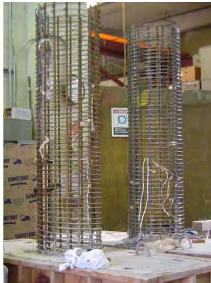
Figure B-34: Completed column cages for DB5-RE (left) and LB8-D2 (right) with beam cast
