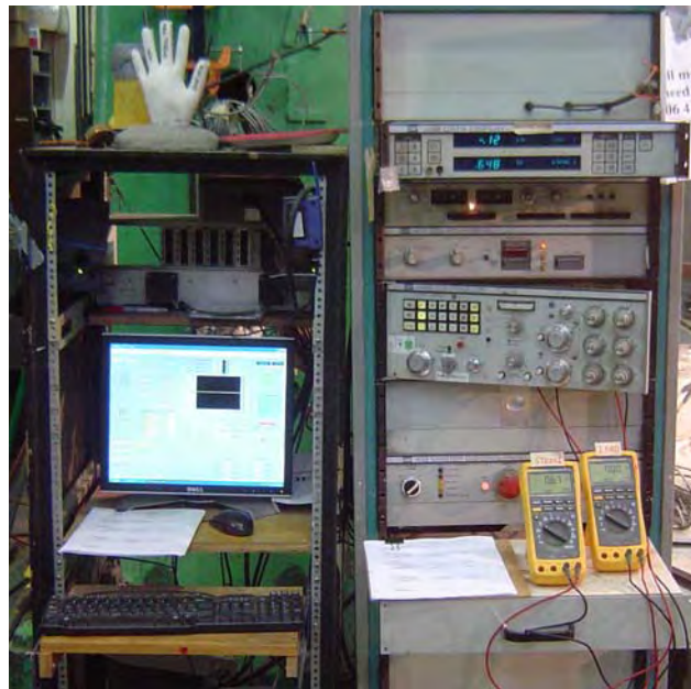
Figure 3-5: Data acquisition system and MTS controller
