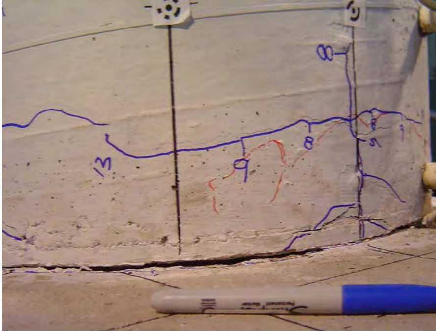
Figure 4-18: Concentrated deformation at the interface in Specimen LB8-FB at Cycle 21 (1.69%/-1.76%)
