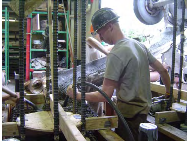
Figure B-30: Casting of specimens LB8-FB and LB8-D1
