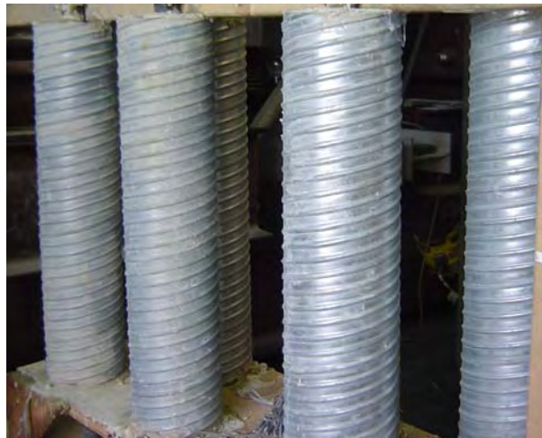
Figure B-18: Corrugated metal ducts used in specimens LB8-FB, LB8-D1 and the pullout tests
