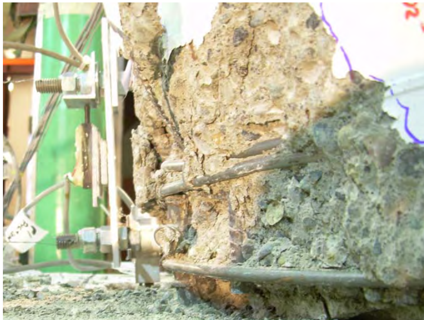
Figure 4-36: Bar 1 buckling in Specimen LB8-D1 during Cycle 32 (5.77%/-5.67%)
