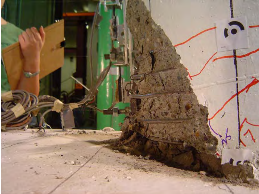
Figure 4-53: Bar 1 buckled in Specimen LB8-D2 at Cycle 32 (5.81%/-5.70%)
