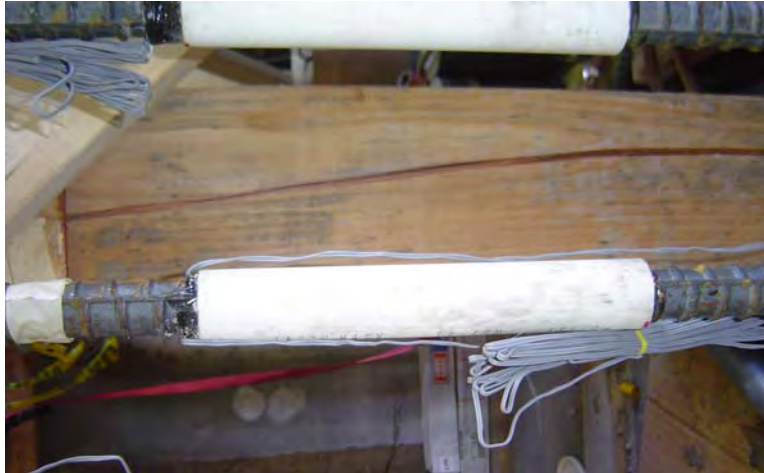
Figure B-21: Debonding of a #8 rebar using Method 2
