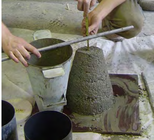
Figure B-13: Slump test conducted before each pour
