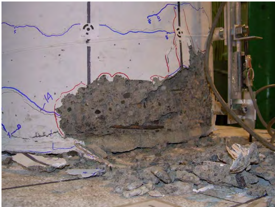
Figure 4-34: Reinforcement exposed in Specimen LB8-D1 Cycle 25 (3.03%/-3.06%)
