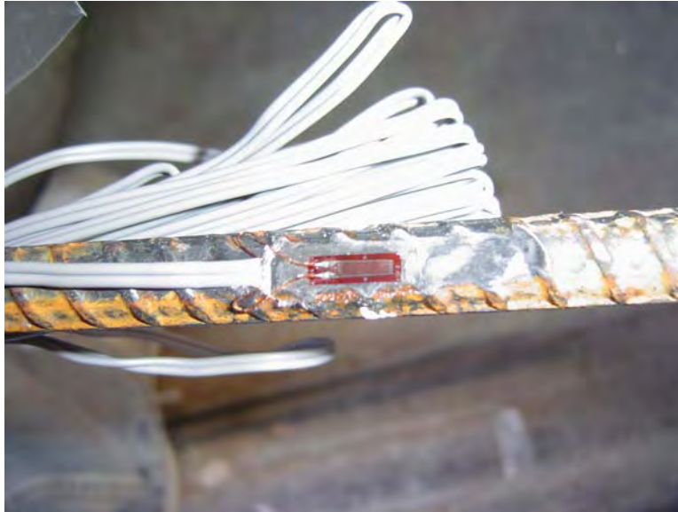
Figure B-23: The area of steel removed from a #3 bar with the strain gage affixed
