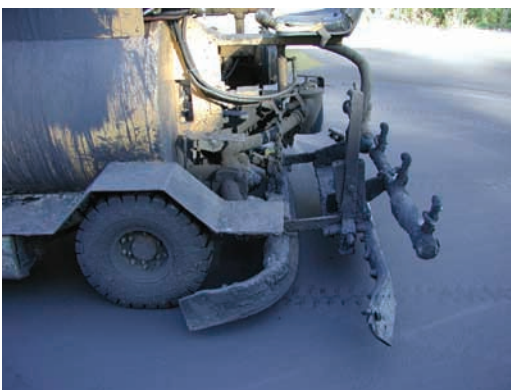
View of squeegee system on sealer applicator.
