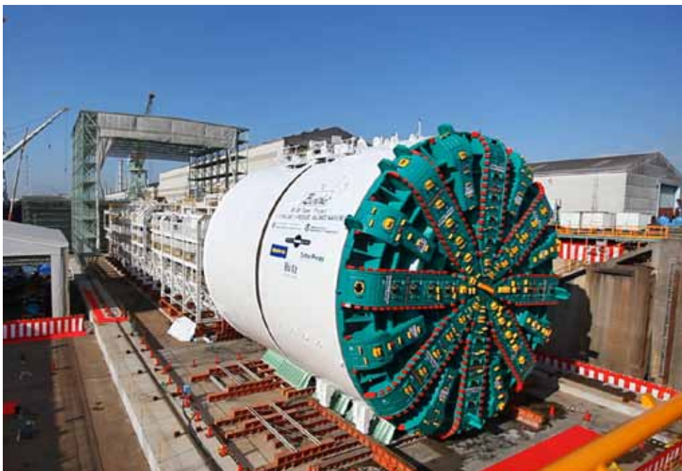
The SR 99 tunneling machine in Japan.
