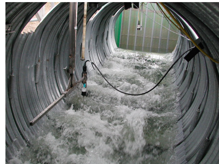
Hydraulic testing of baffles in 2006.
