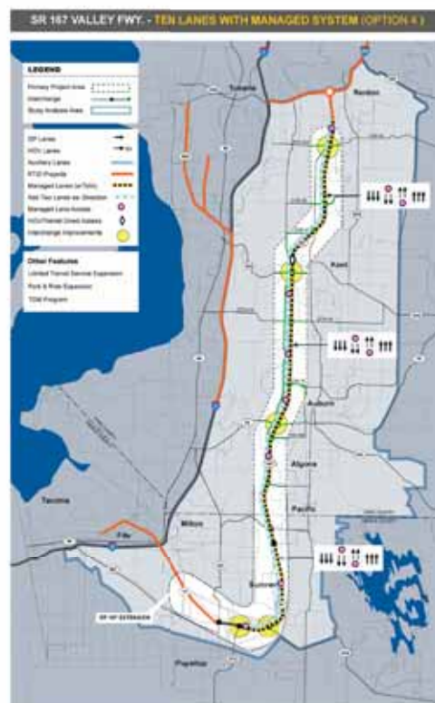
Option 4 provides four new general-purpose lanes, a new HOV-only ramp, and interchange upgrades along the corridor. May be a managed lane system.
