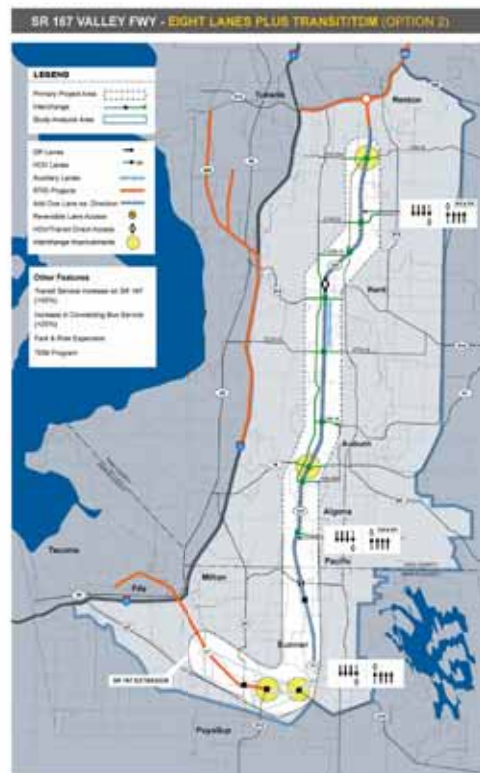
Option 2 provides an expanded transit service a less aggressive TDM plan, two new general-purpose lanes, and a reversible managed lane
