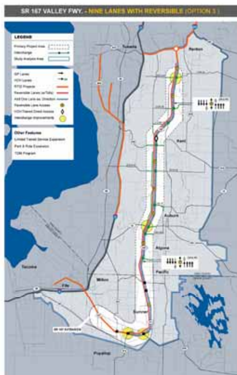
Option 3 provides two additional general-purpose lanes and a reversible managed lane.
