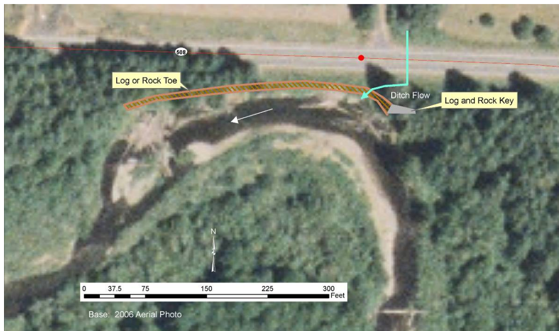
Figure 13. Extent of Toe Treatments (Alternatives 2 and 3).
