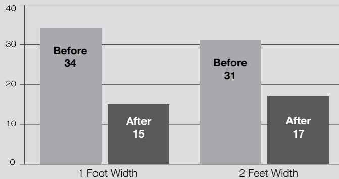
Number of Crossover Crashes on U.S. 12 between Tri-Cities and Walla Walla After Installation of Center Line Rumble Strips
