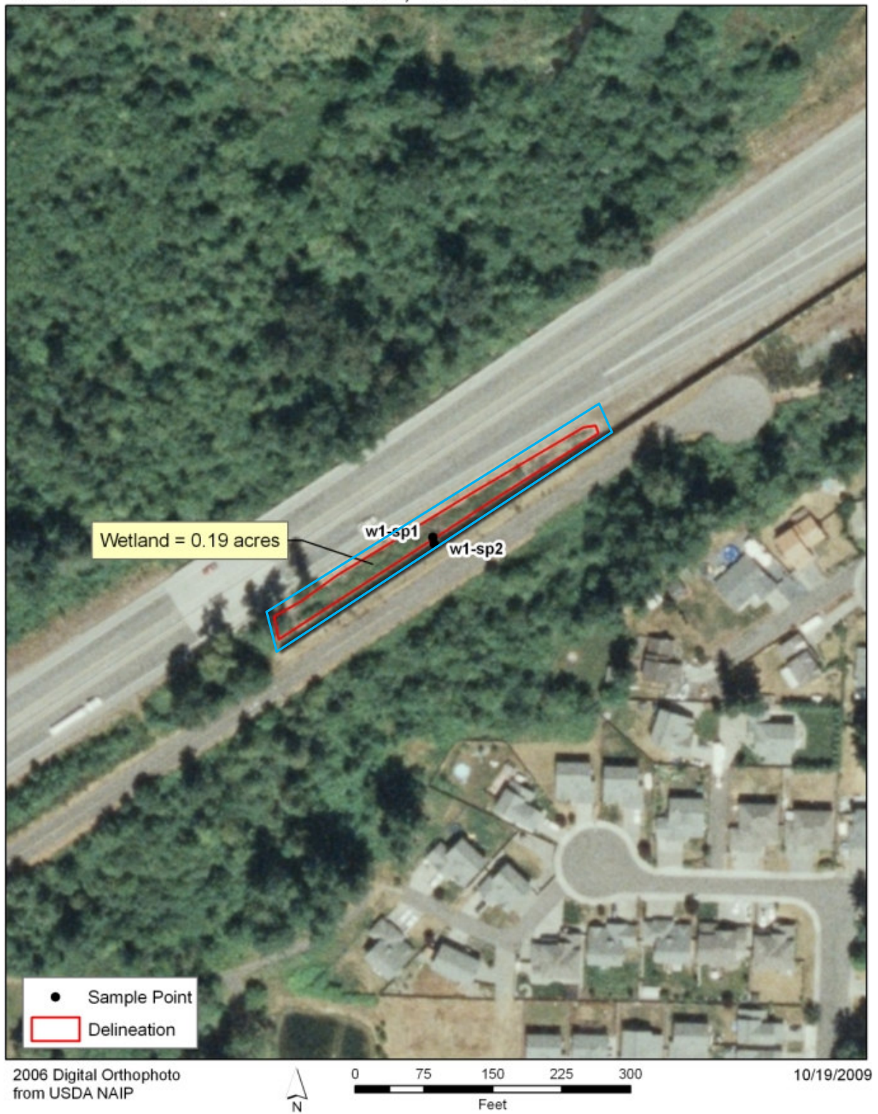
Figure 2. Study area shown in blue, wetland boundary shown in red, sampling point locations shown in black.
