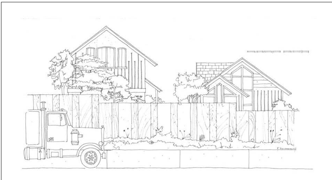
Example of community scale wood wall 6 to 8 ft high. Dashed line above roof on the right shows typical noise wall height at 14 ft.
