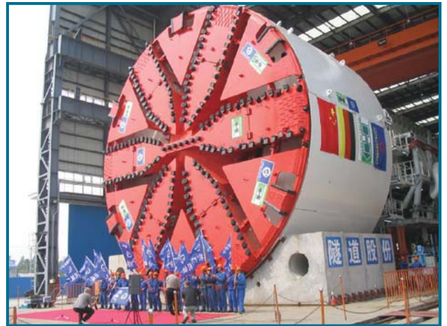
This tunnel boring machine is 50.6 feet in diameter and is similar in size and type to the machine we would use to build the proposed SR 99 bored tunnel.
