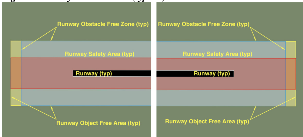
Figure ? Runway Critical Areas (typical)
