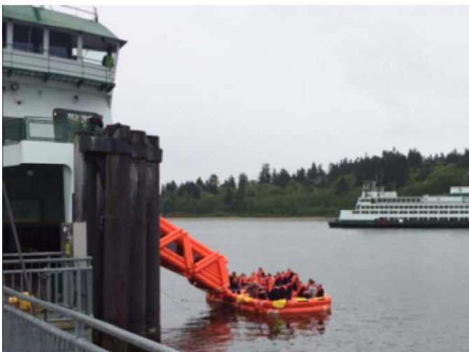
Life raft testing in May on the Salish. The passenger evacuation slides with life rafts are tested every six years.
