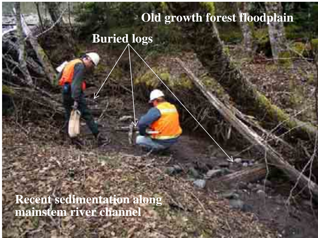
Another example of buried log matrix beneath old growth floodplain forest along right (East) side of river near MP 51. April 25, 2005.
