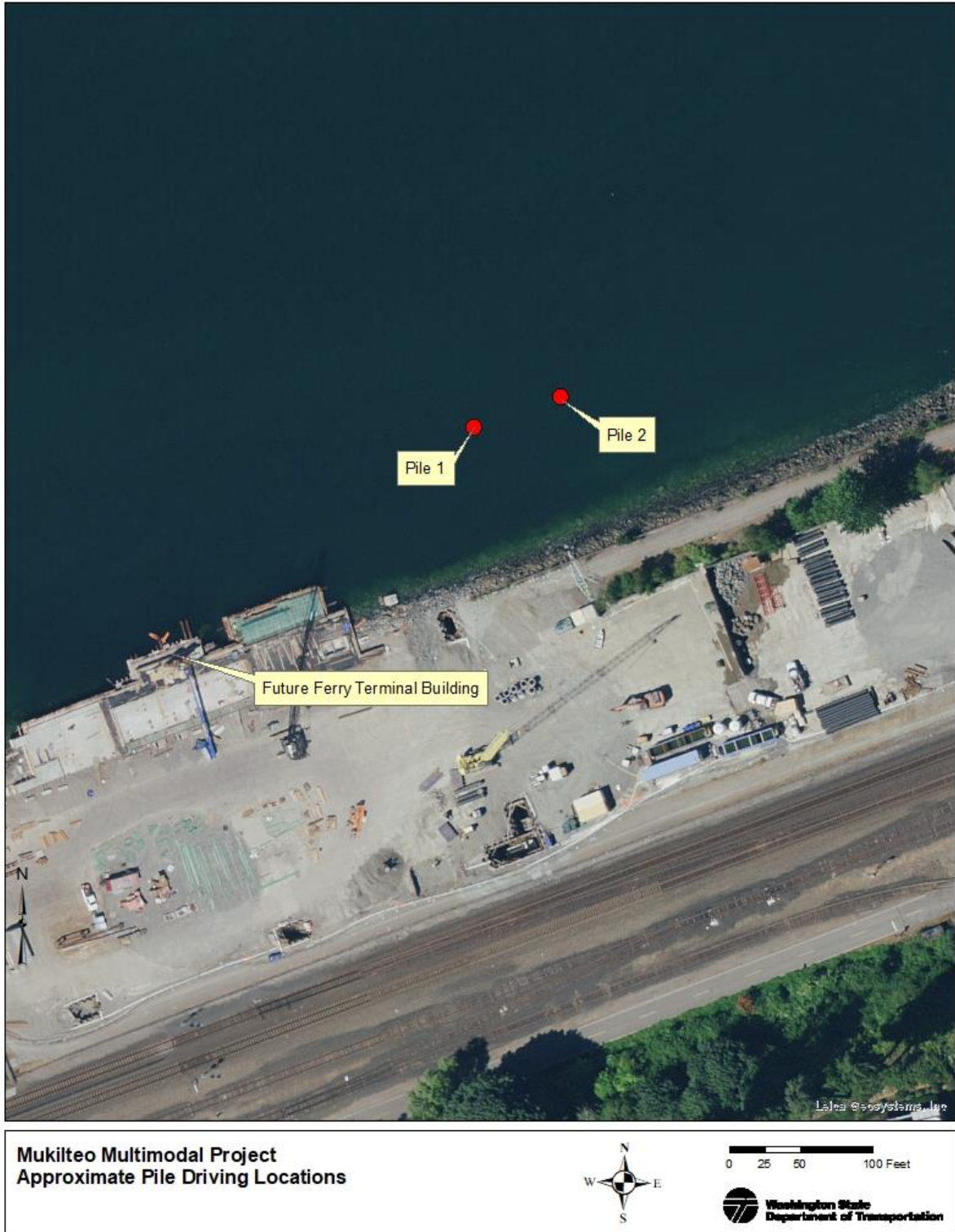
Figure 3: Approximate Locations of Piles 1 and 2 at Mukilteo Ferry Terminal (Phase 3) Project
