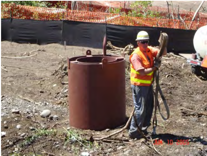
Figure 7: Confined bubble curtain for use in shallow waters with swift currents.
