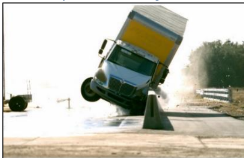
Photo C: Box Truck Leaning Over High Performance Barrier During Impact
