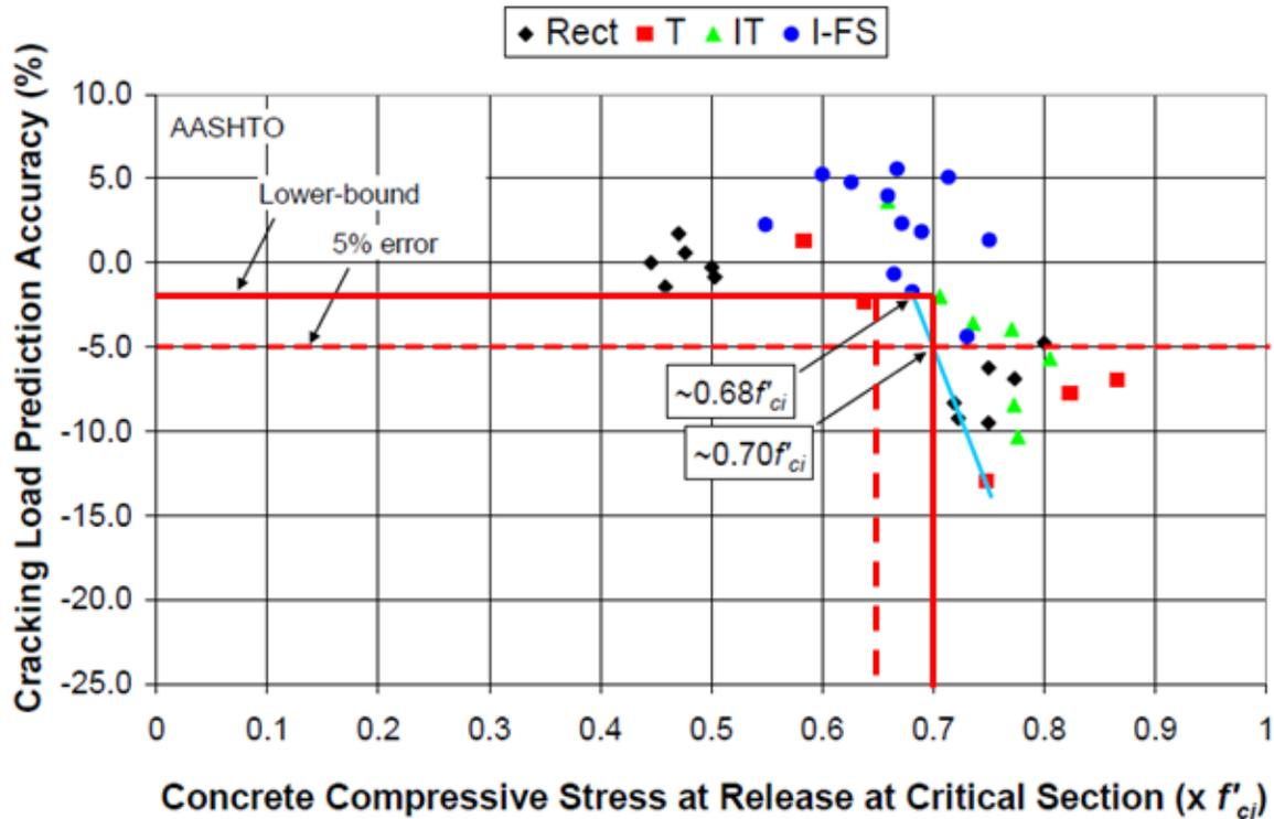
According to descriptions of relevant research provided in Birrcher, et. al. [2], the  $0.65f'_{ci}$  recommendation was based on tests of specimens that were either uniformly loaded in compression or did not have lateral bending concerns as noted above. Therefore, the experimentation represents a “global” stress condition in the specimens. Bending about the minor axis does not result in a net change in these “global” stresses, but introduces peak stresses at the extremities of the member.
