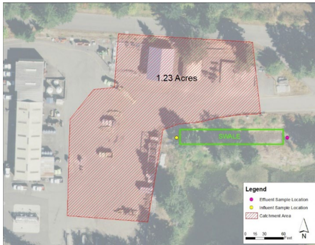
Figure 2. Mottman CABS monitoring site and associated drainage
