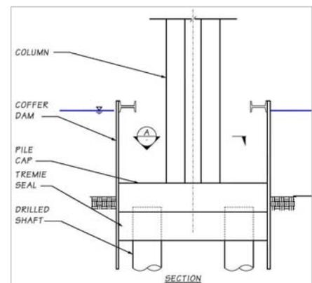
Cross Section of Drilled Shaft Cap and Column Configuration
