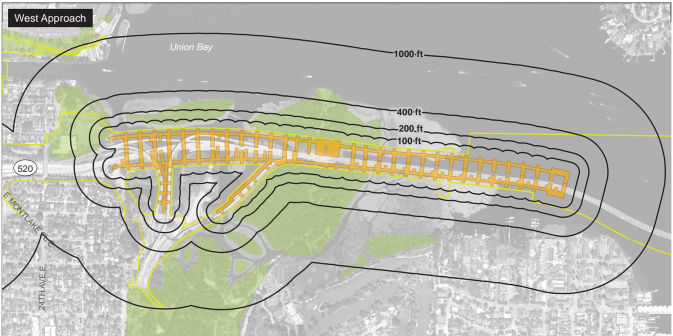
Note: Pile-driving activities and locations would be similar for the Preferred Alternative and Options A, K, and L. Predicted Pile-Driving Noise Levels versus Distance (worst case noise levels based on 105 dB max at 50 feet with no additional shielding attenuation) pile-driving noise would occur only for limited durations during the construction period, and would be required to meet the noise control ordinance or have a variance.
