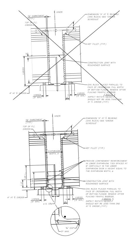
End Type C (Intermediate Hinge Diaphragm) Figure 5.6.2-5
