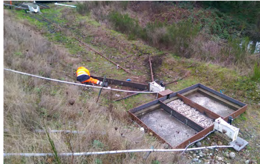
Figure 7. WSDOT monitoring staff setting up the Lakeview bioswale for future monitoring studies.
