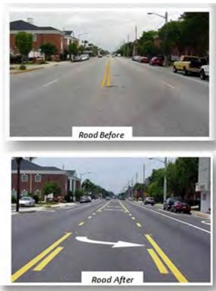
FIGURE 10. ROAD RECONFIGURATION. SOURCE: FHWA.
