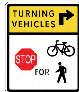
FIGURE 33. MODIFIED R10-15 SIGN
