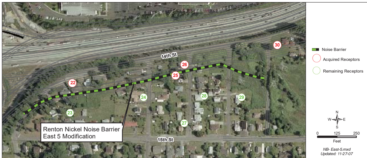
Exhibit 6-2: Renton Nickel Noise Barrier East 5 Modification
