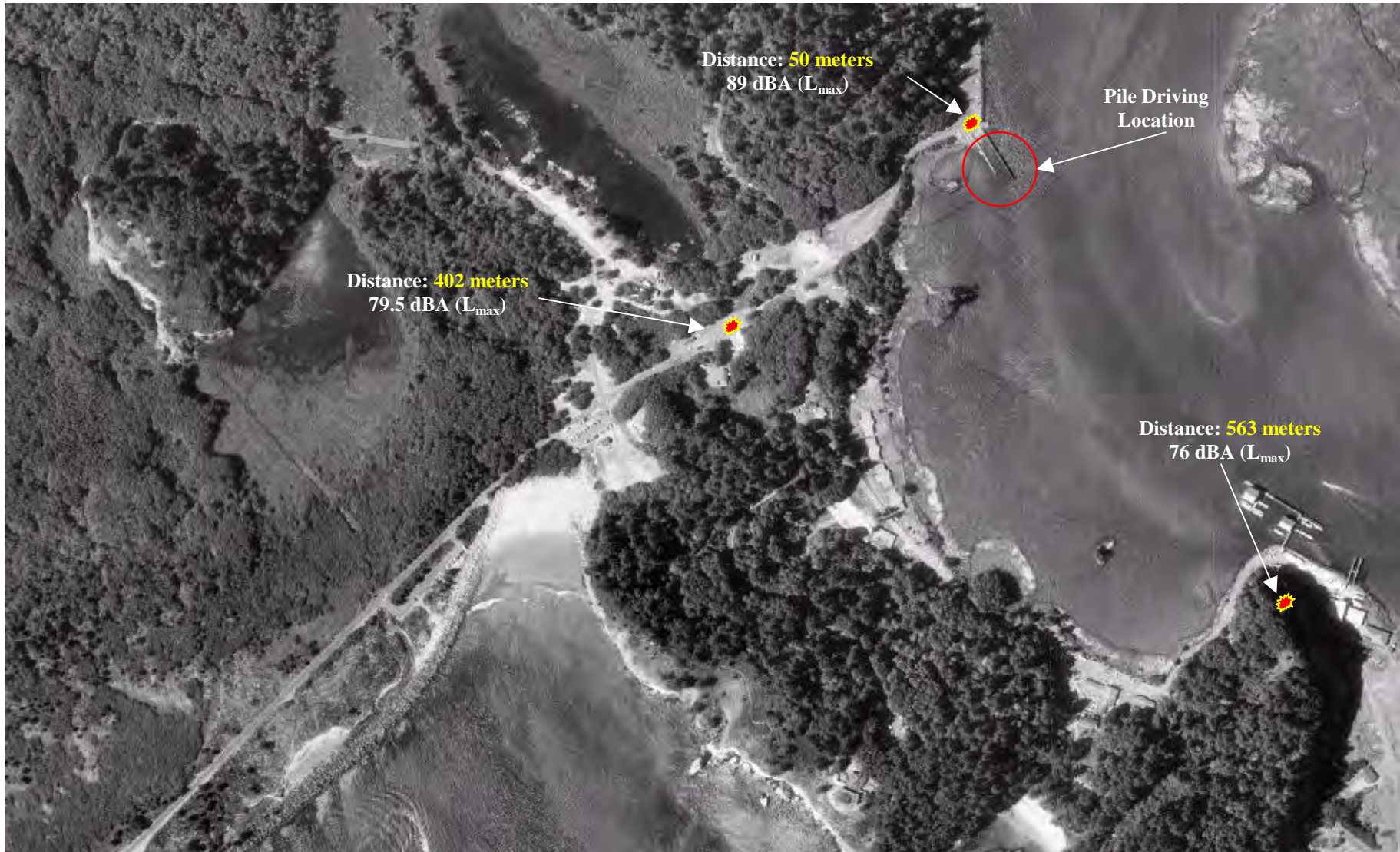
Figure 11: Airborne measurement locations (☀) with A-weighted maximum values.
