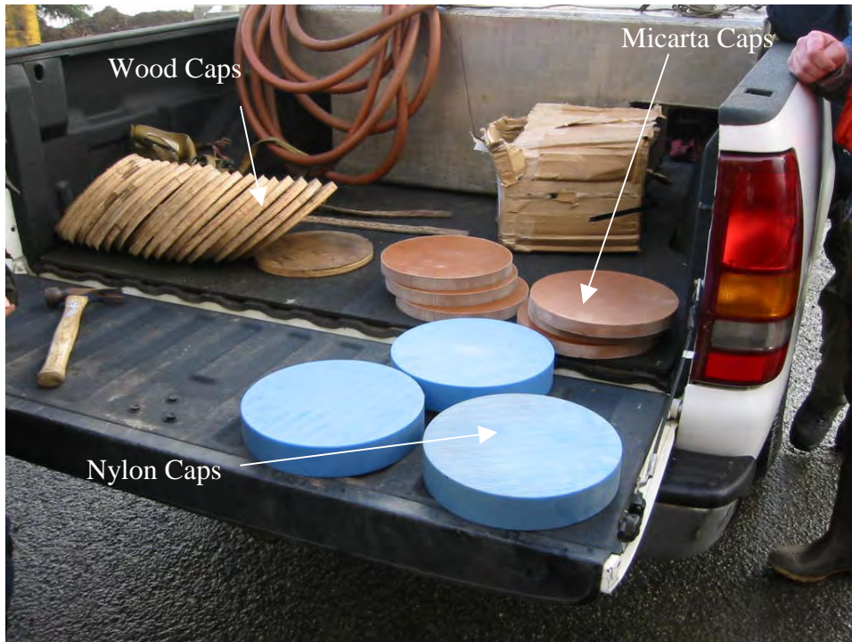
Figure 1: Pile cap types tested in this monitoring project (Conbest pile cap not shown).
