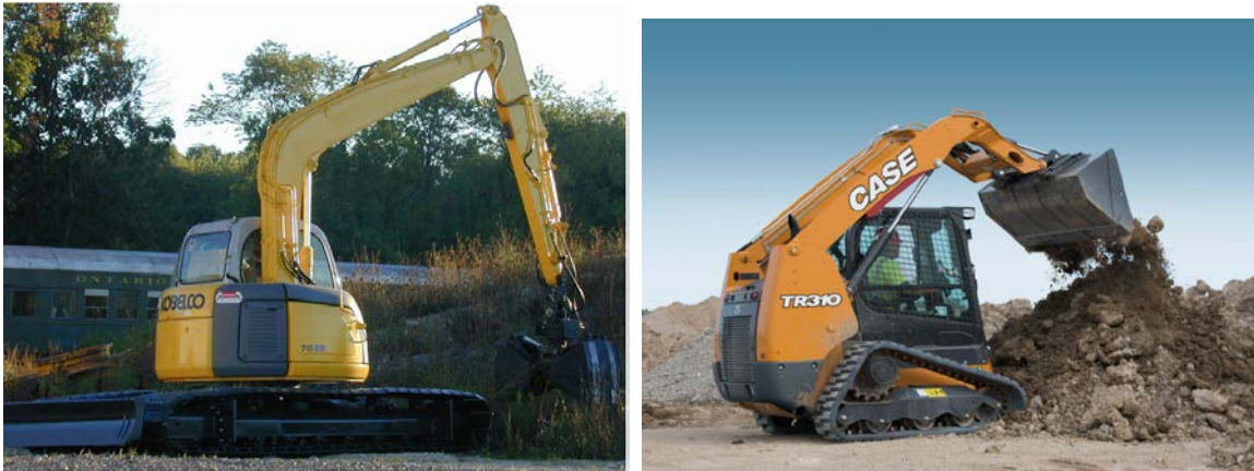
Exhibit 6: Examples of 4-5 psi ground pressure equipment.
