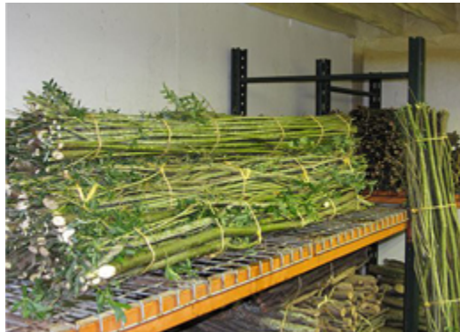
Exhibit 12: Live Fascines ready for installation.
