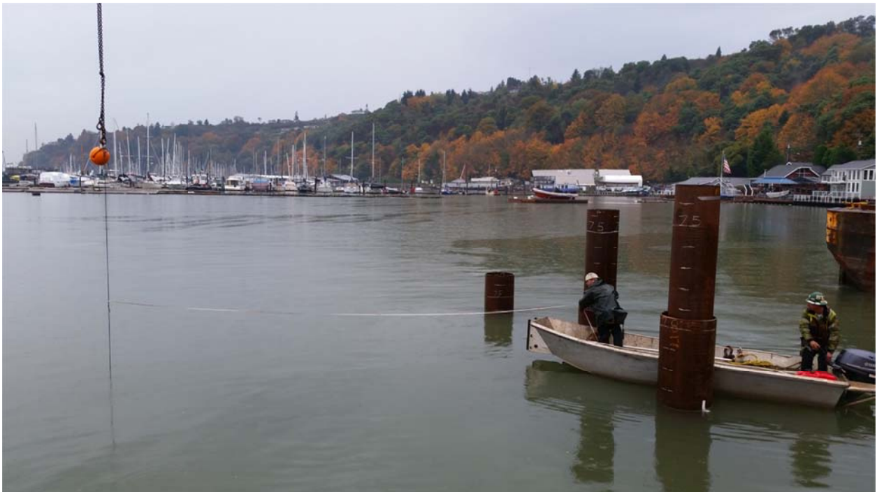
Figure 3b. Photograph made on October 30 th of the 3 piles shown in order of nearest to farthest: Mandrel Pile, Double Pile and Control Pile. The VLA, now under tension is shown on the left while its range from the piles is measured.
