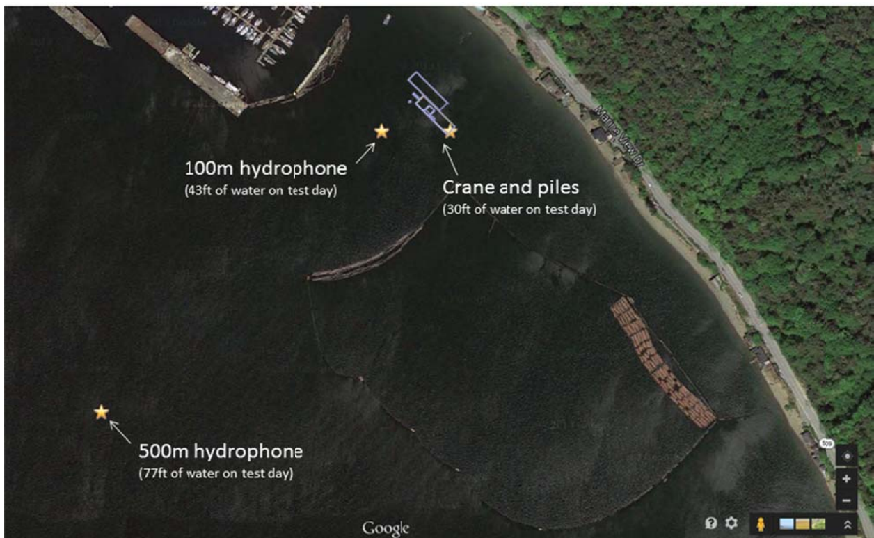
Figure 6. Notional position of the 500 m hydrophone with respect to the pile sources (see text for exact range from piles.)
