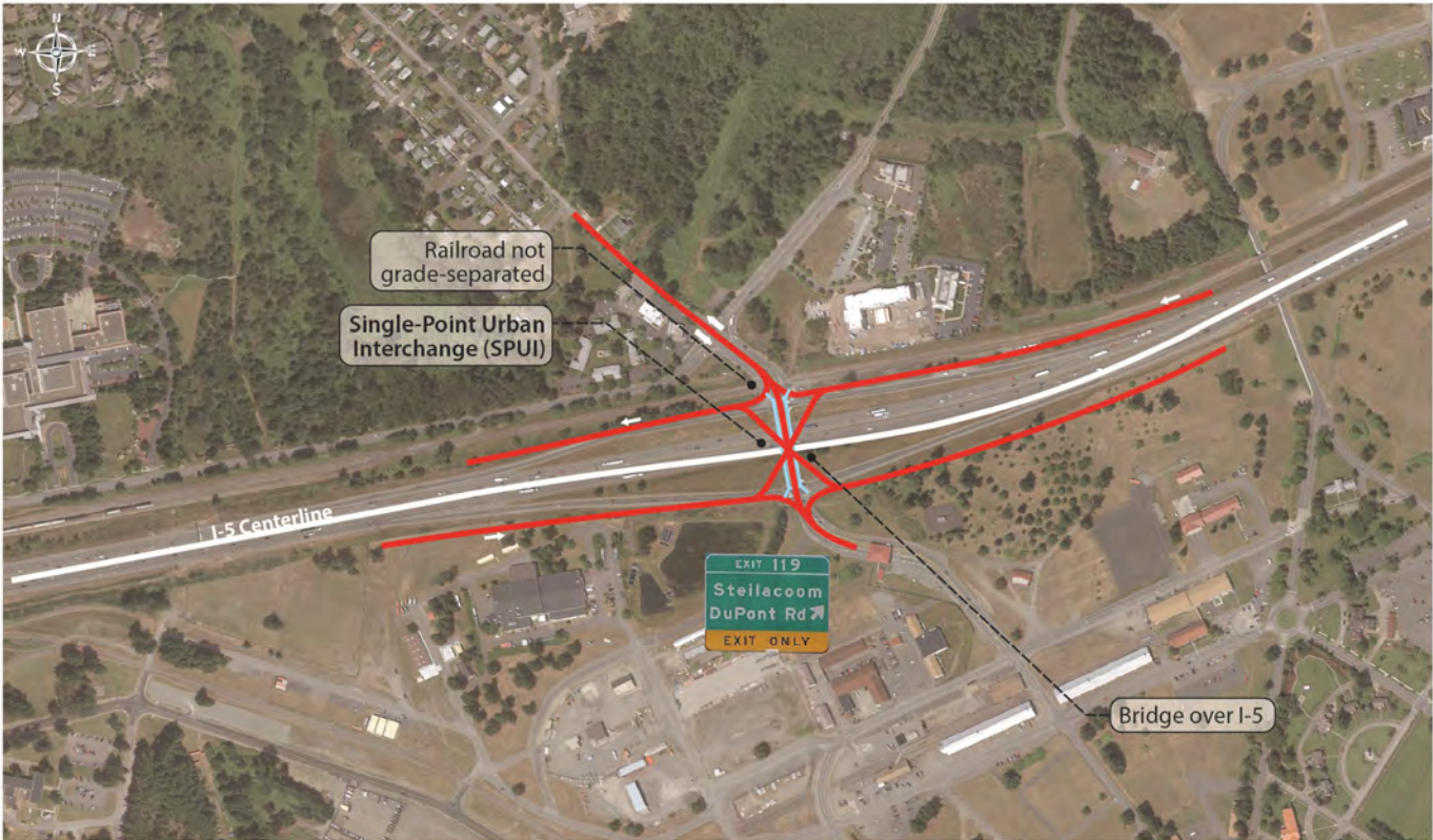
Figure VII-4: Steilacoom-DuPont Interchange - Concept C – Single Point Urban Interchange (SPUI)
