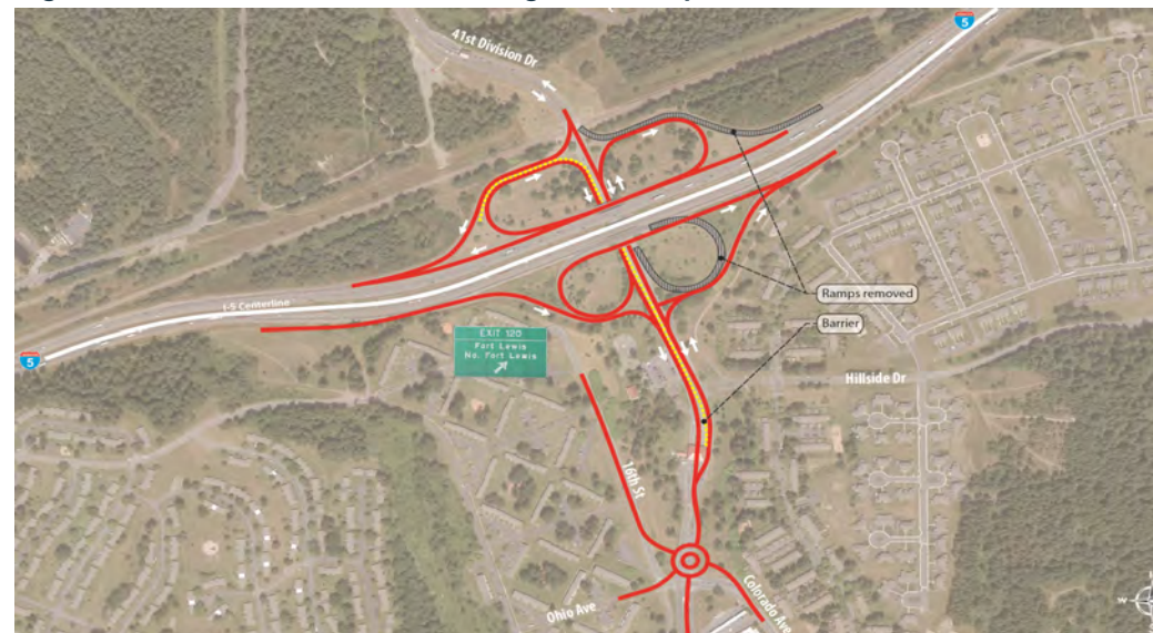
Figure VII-16: Thorne Lane Interchange - Concept D – Relocated Tight Diamond Interchange
