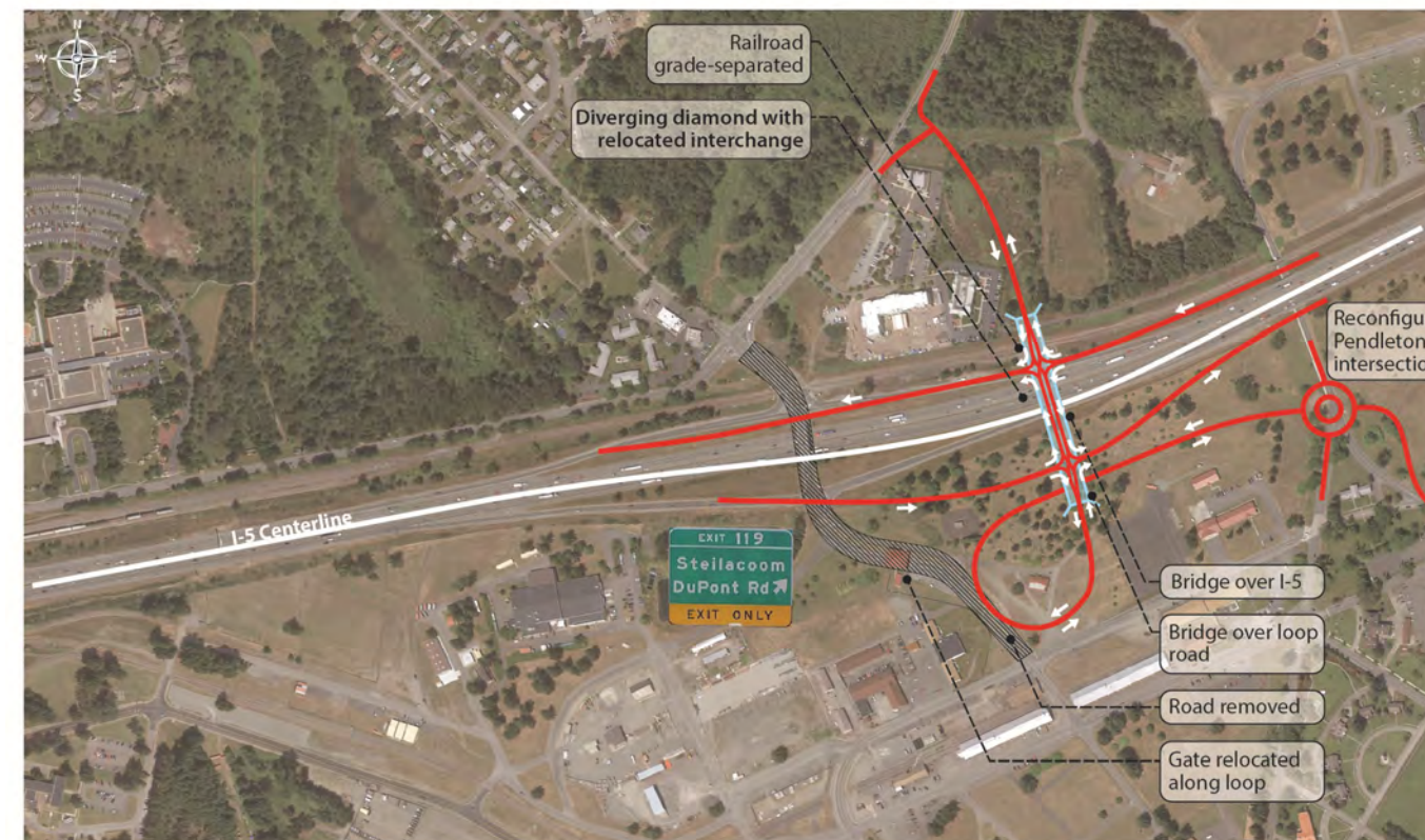
Figure VII-2: Steilacoom-DuPont Interchange - Concept A – Offset Diverging Diamond Interchange
