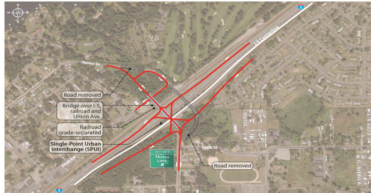
Figure VII-13: Thorne Lane Interchange - Concept C – Offset Single Point Urban Interchange (SPUI)
