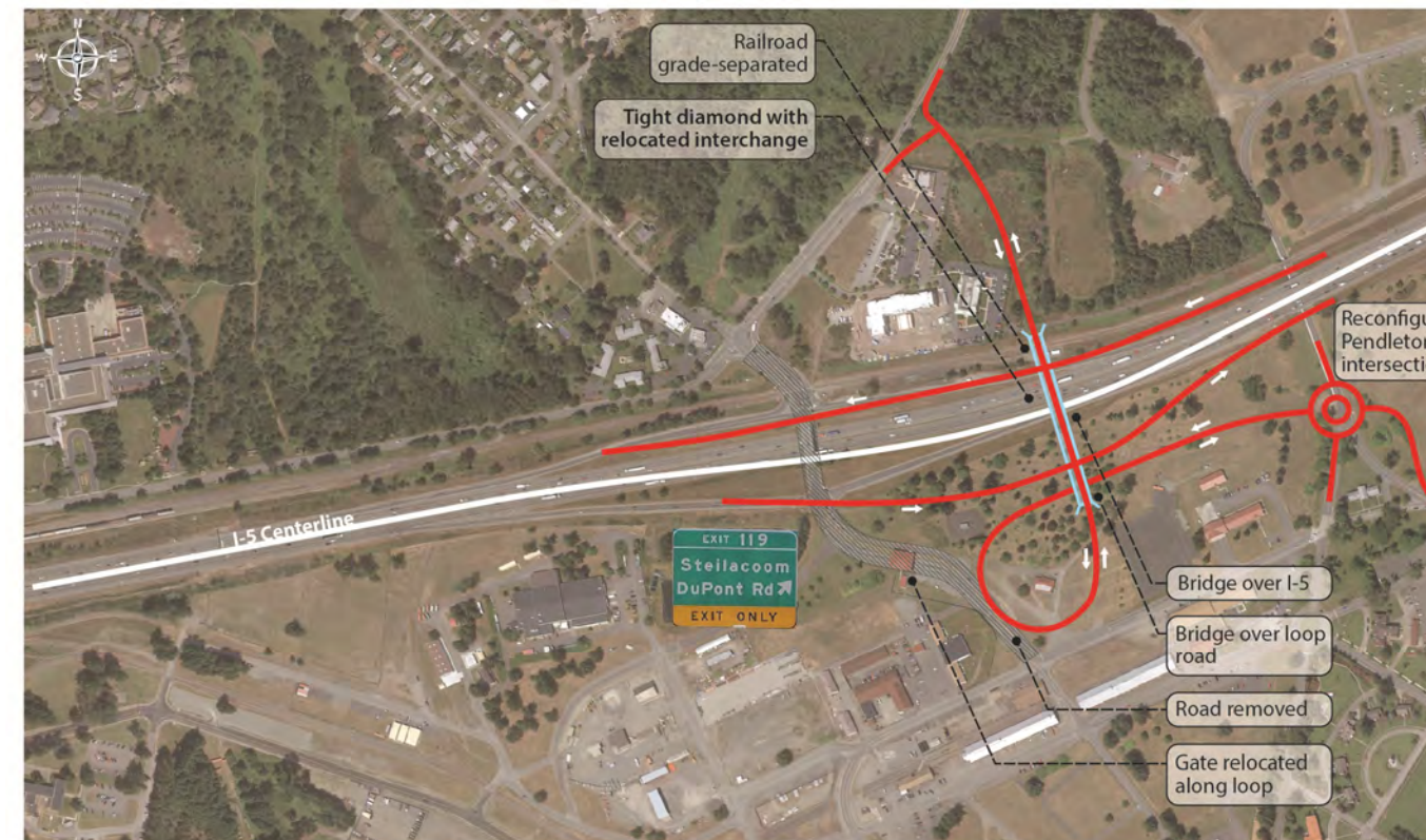
Figure VII-3: Steilacoom-DuPont Interchange - Concept B – Offset Tight Diamond Interchange
