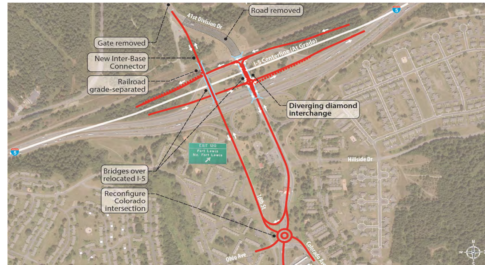
Figure: VII-6: Main Gate Interchange - Concept B – Diverging Diamond Interchange with Realigned I-5 and Inter-Base Connection
