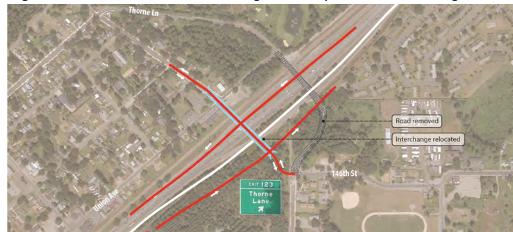
Figure VII-16: Thorne Lane Interchange - Concept D – Relocated Tight Diamond Interchange
