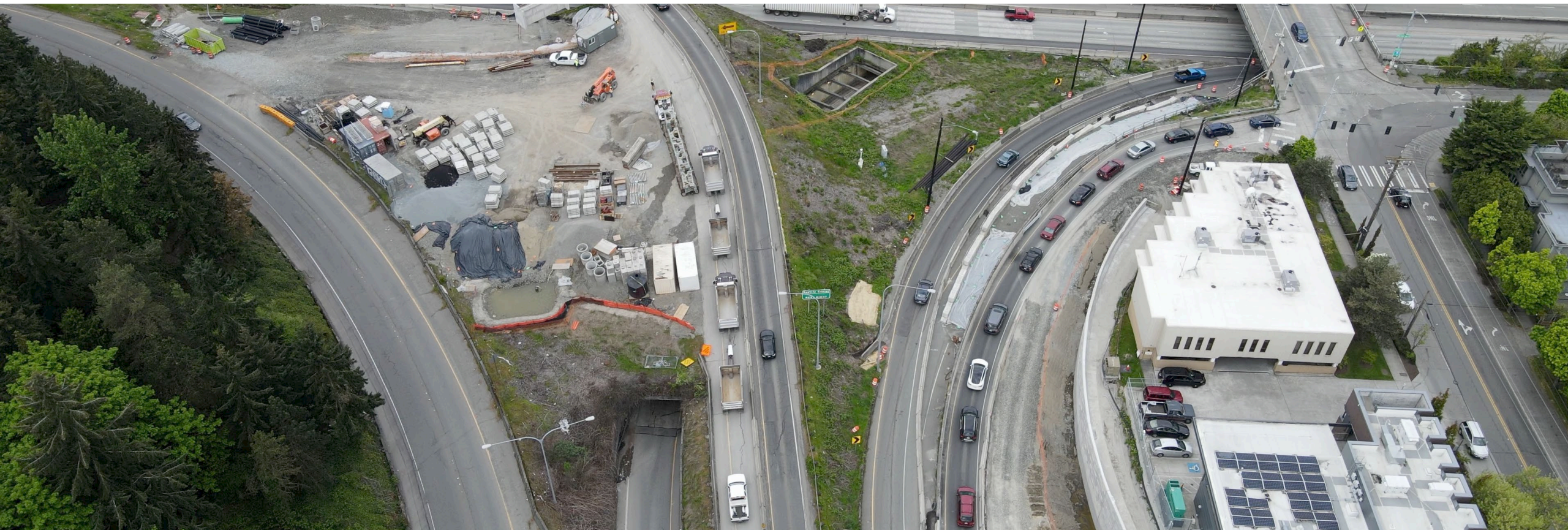
From above, the westbound SR 520 off-ramp to Roanoke St. and northbound I-5 will soon be "pushed" north (right in photo) to make room for new flyover ramp
