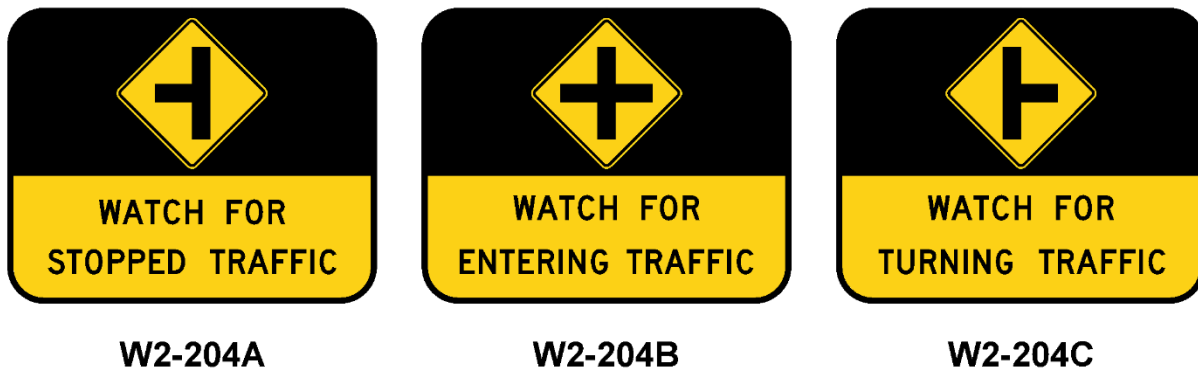
Exhibit P2.7-5: Major Roadway ICWS Enhanced Signs – W2-204 Series
